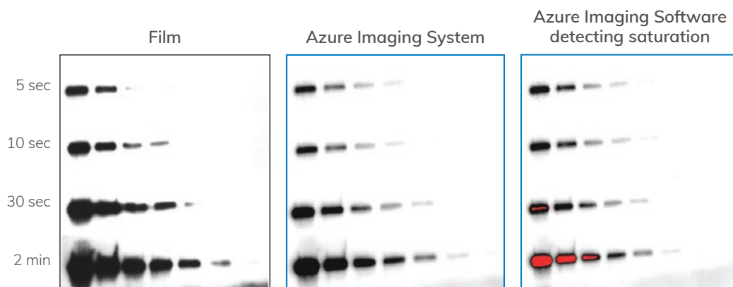
Figure 1. Saturation detection prevents errors in quantitation. The same Western Blot was imaged on both x-ray film and the Azure Imaging System. The Azure system detects when CCD saturation occurs and calculates an auto-exposure time to avoid saturated bands.
