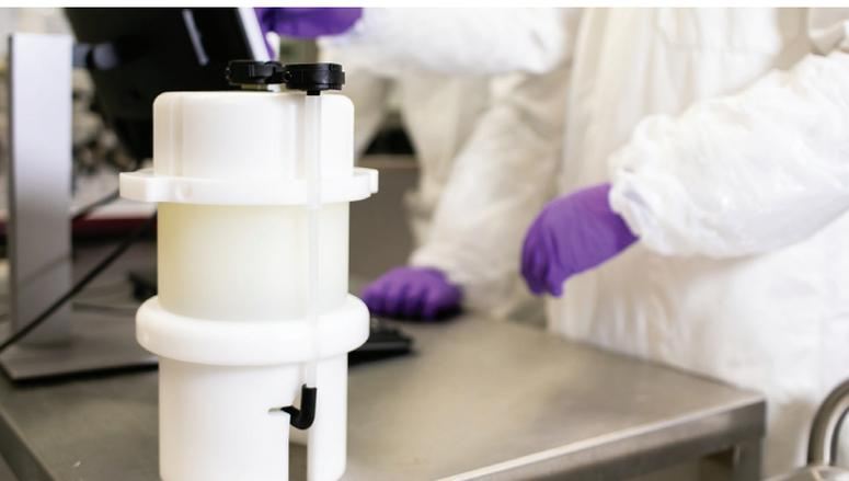
Evolve®D Process columns are supplied qualified and ready for use, pre-packed with chromatography media from the Astrea Bioseparations range of products for applications such as protein purification and contaminant removal. The columns can also be custom packed with a range of media types including agarose & polymethacrylate based adsorbents.
