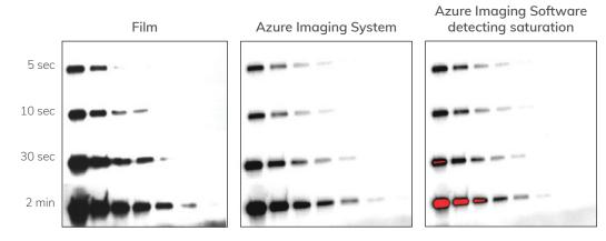
Figure 1. Saturation detection prevents errors in quantitation. The same Western Blot was imaged on both x-ray film and the Azure Imaging System. The Azure system detects when CCD saturation occurs and calculates an auto-exposure time to avoid saturated bands.
