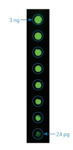
Figure 12. Two-fold serial dilutions of AzureSpectra-800 labeled antibody were spotted on a nitrocellulose dot-blot, and imaged in the 800nm channel for 20 seconds.
