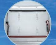
Safety lid with unbreakable, robust platinum electrodes, flexible positioning
